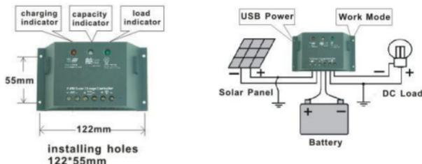
1. Check whether the installing place accords with safety stipulation. Avoid installing the controller in such place as wet, flammable, explosive places and places with corrosive gas.
