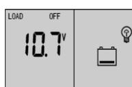
As shown on the left, shows the values of LVD voltage. When the battery voltage is lower than protection voltage, the controller will disconnect the load circuit to prevent battery over-discharge.
