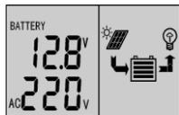
As shown on the left, displays charge status, battery status, voltage of battery, voltage of AC output, wind turbine and grid power status.
