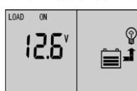
As shown on the left, shows the values of LVR voltage. Under the LVD protection in the controller, when the battery voltage is restored to the higher voltage than LVR voltage, the controller will re-connect the load circuit. In this interface you can use the button 、 to adjust the parameter. The number will be flash. After long press the key (> 5seconds) , the number will be saved and stop flash. Short press to give up save the number and exit to next interface.
